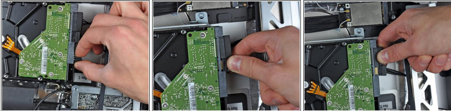
**⚠** Before disconnecting the thermal sensor cable, take note of its orientation. It is extremely important to reinstall the connector in the current orientation so the fans will not run at full speed. If you have multiple pins on your replacement hard drive, put the connector closest to the SATA connections and closest to the PCB board.
